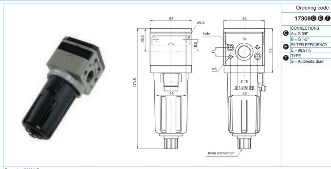
Example: 17308A.E Coalescing filter size 3 with G 3/8" connections and filter efficiency of 99,97%
