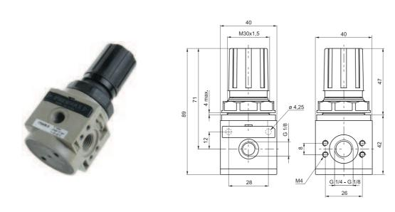
Ordering code 17**Ø**02**@**.**@**. VERSION 0 = Zinc alloy body 1 = Technopolymer body CONNECTIONS **e** A = G 1/8" B = G 1/4" ADJUSTING RANGE A = 0 - 2 bar**G** B = 0 - 4 barC = 0 - 8 bar D = 0 - 12 bar TYPE L = no Relieving SM = improved relieving
