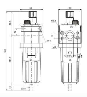
Ordering code 17203**©**. CONNECTIONS A = G 1/4" B = G 3/8" TYPE MA = Min. oil level indicator N.O. MC = Min. oil level indicator N.C.
