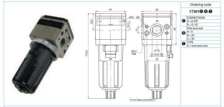
Example: 17301A.B Filter size 3 with G 3/8" connections and filter pore size 20
